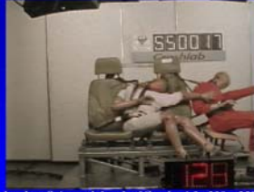
Richardson S.A., et al, Int. J. of Crash , 4:3, 239 - 259, 1999 Side facing 4-point harnesses demonstrated to be lethal, even at slow ground vehicle speeds
