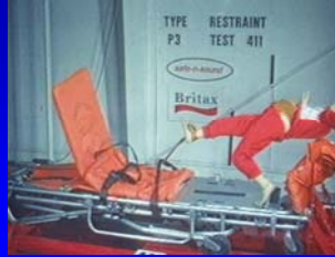
Levick NR, et al. Development and Application of a Dynamic Testing Procedure for Ambulance Pediatric Restraint Systems, SAE Australasia 1998;862:45-51
