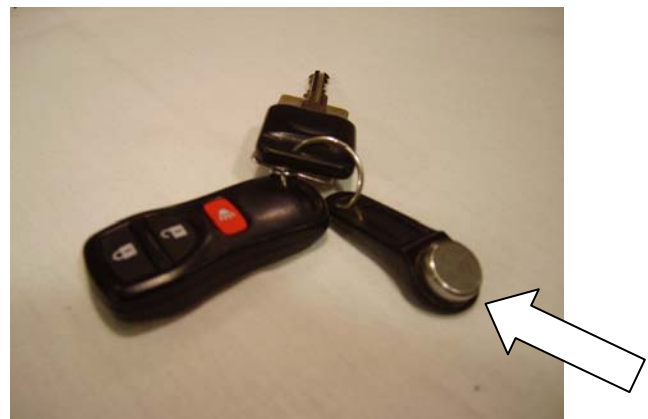
Figure 1. Key fob for the EMS vehicle driver to engage onboard monitoring and feedback device
