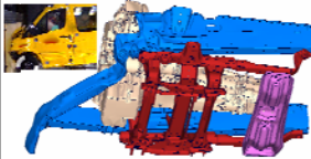
Front axle module after crash
